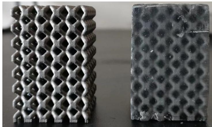
**Figure 4.** Fabrication of 316L metallic lattice structure and epoxy/316L metallic lattice structure.
