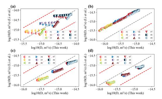
**Figure 3.** Comparison between the interdiffusion coefficients of different diffusion couples (noted with #1–#3 for 1273 K and 48 h, #4–#6 for 1323 K and 48 h, and #7–#9 for 1373 K and 48 h, evaluated by Li et al. [20] as listed in Table 1) and optimization results in the present work: (a)  $\tilde{D}_{AlAl}^{Ni}$ ; (b)  $\tilde{D}_{CoCo}^{Ni}$ ; (c)  $\tilde{D}_{CrCr}^{Ni}$ ; (d)  $\tilde{D}_{FeFe}^{Ni}$ .
