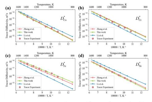
**Figure 4.** Comparison between the tracer diffusion coefficients evaluated by different researchers [20,24,35] and optimization results in the present work: (a)  $D_{Co}^*$ ; (b)  $D_{Cr}^*$ ; (c)  $D_{Fe}^*$ ; (d)  $D_{Ni}^*$ .
