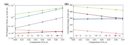
**Figure 7.** Influence of aluminum content on (**a**) pre-frequency factors and (**b**) activation energies of the tracer diffusion coefficients of the Alx(CoCrFeNi)1-x alloys.
