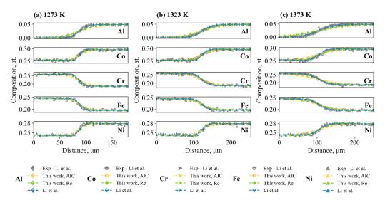
**Figure 2.** Comparison of the typical composition profiles among the experimental results (Li et al. [20]) and model-predicted results due to Li et al., optimization with parameter selection based on AICc and optimization with regularization based on L2 norm penalty: (**a**) 1273 K; (**b**) 1323 K; (**c**) 1373 K.
