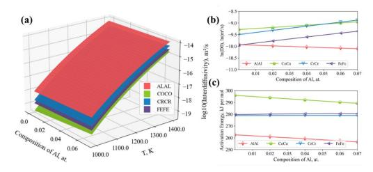
**Figure 5.** Influence of aluminum content on the main terms of the interdiffusivity matrices of the Alx(CoCrFeNi)1-x alloys: (**a**) Surface plot for interdiffusivites; (**b**) Pre-frequency factors of Arrhenius relation; (**c**) Activation energies of the Arrhenius relation, where ALAL stands for  $\tilde{D}_{AlAl}^{Ni}$ , COCO for  $\tilde{D}_{CoCo'}^{Ni}$  CRCR for  $\tilde{D}_{CrCr}^{Ni}$  and FEFE for  $\tilde{D}_{FeFe}^{Ni}$ .
