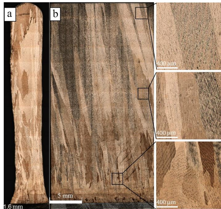
**Figure 7.** Profile (a) and front (b) cross section optical views of Cu-3wt.%Si-Mn bronze wall obtained at heat input of 0.31 kJ/mm with enlarged insets representing the bottom, medium, and top parts of the wall.
