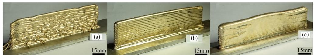
**Figure 2.** Optical images of thin walled samples obtained at heat input levels 0.19 kJ/mm (a), 0.21 kJ/mm (b), and 0.31 kJ/mm (c) (Table 1).
