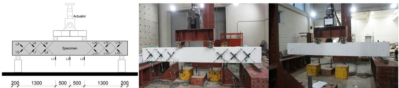
**Figure 4.** Loading test configuration [unit: mm].
