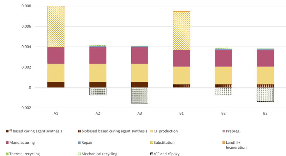
**Figure 4.** Impact contribution for the 6 scenarios across each life cycle of the FU for the *Global Warming* impact category. Negative impact values of *rCF* and *rEpoxy* are due to the avoided impact of virgin CF and epoxy resin because of their recycling. The quantitative avoided impacts are related to the chosen recycling option and its efficiency of recovery.
