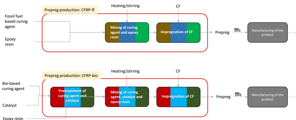
**Figure 2.** Prepreg production process on a laboratory scale. CFRP-ff (i.e., group of scenario A) includes two main steps: firstly, mixing the dynamic curing agent with the epoxy resin, and secondly, the impregnation of the CF. CFRP-bio (i.e., group of scenario B) includes the same steps of scenario A plus two additional pretreatment steps needed for the dynamic curing agent and catalyst. Colors represent the different scenarios.
