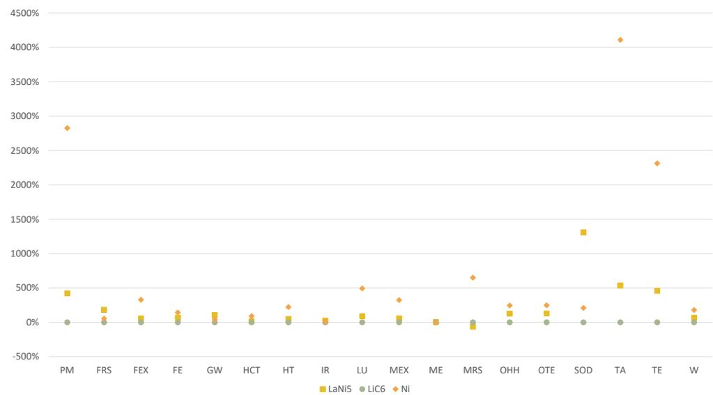
**Figure 7.** Sensitivity analysis on mechanical recycling. According to different providers of electrode production, some of the impact categories are affected by the results. Compared to LiC6, which is the base case, the highest and the lowest variability is observed, respectively, for *Terrestrial acidification* and *Marine eutrophication* categories.
