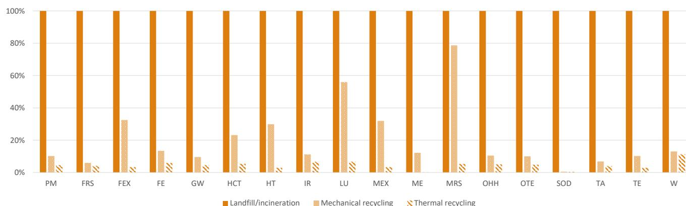
**Figure 6.** Comparative LCA between EoLs of composites. Incineration and landfill are representative of the most common composite waste management and hence are the baseline of the analysis. Relevant reduction in all the impact categories both for the thermal and mechanical recycling pathways. Limited environmental benefits compared to the baseline are shown for mechanical recycling in *Mineral resources scarcity*.
