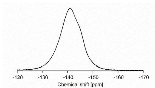
**Figure 2.**  $^{19}\text{F}$  CP MAS NMR spectra of HHU-COF-2.
