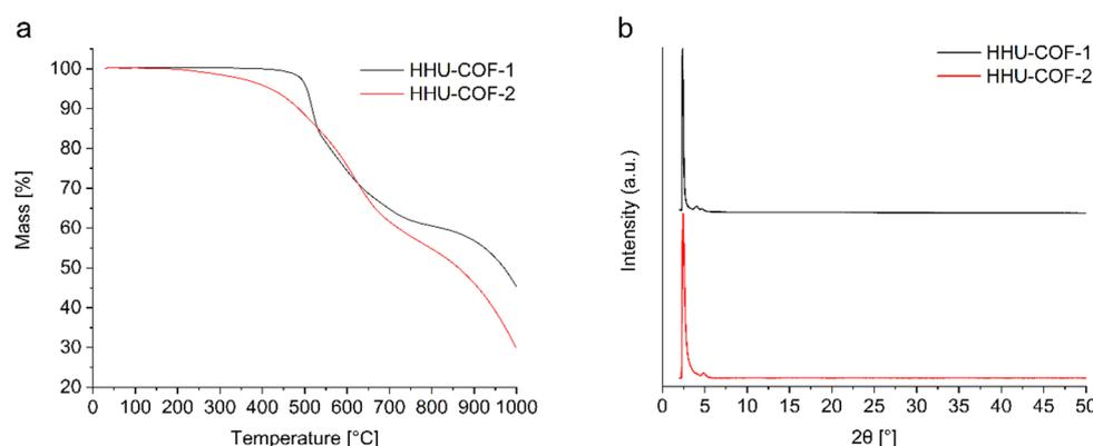
**Figure 5.** (a) TGA curves acquired under nitrogen atmosphere with a heating rate of 5 K/min and (b) PXRD pattern of HHU-COF-1 and HHU-COF-2. The first derivative of the TGA curves is given in Figure S15.
