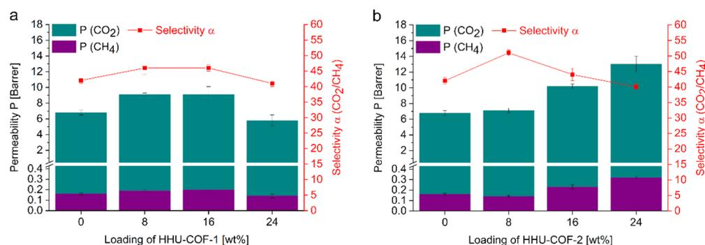
**Figure 8.** CO<sub>2</sub> and CH<sub>4</sub> permeabilities (P) and CO<sub>2</sub>/CH<sub>4</sub> selectivity( $\alpha$ ) for (a) HHU-COF-1/Matrimid and (b) HHU-COF-2/Matrimid MMMs.
