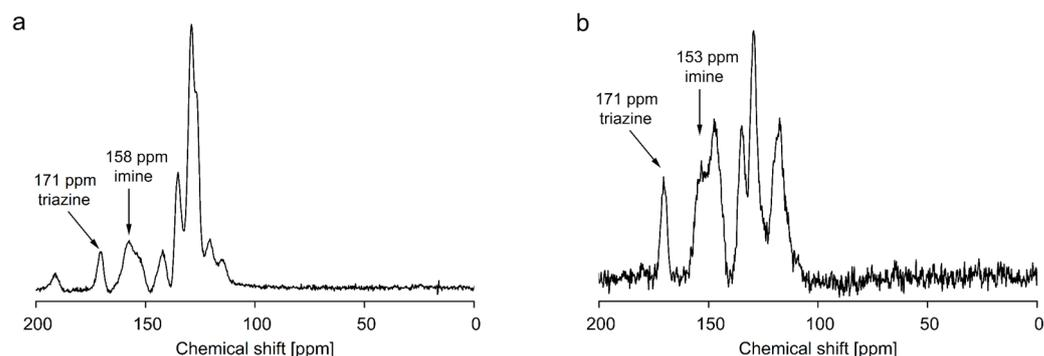
**Figure 1.**  $^{13}\text{C}$  CP MAS NMR spectra of (a) HHU-COF-1 and (b) HHU-COF-2. Spectra were obtained at 150 MHz, cross-polarization with decoupling spinal and 35 kHz spinning.
