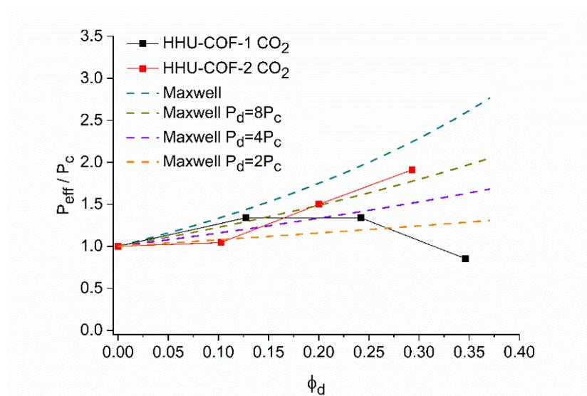
**Figure 10.**  $P_{eff} / P_c$  of the gas CO<sub>2</sub> versus  $\phi_d$  for 0 to 24 wt% HHU-COF-1 and HHU-COF-2 as dispersed phases in Matrimid matrices.
