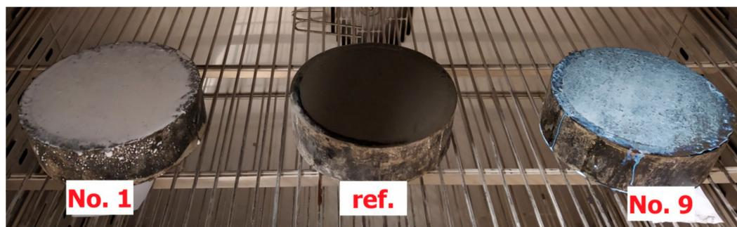
**Figure 2.** Samples of mortar cured in the oven (reference sample and No. 1 and 9).
