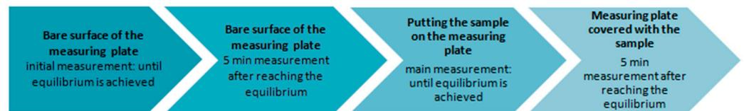
**Figure 2.** Scheme of testing the nonwoven inserts with PCMs on a “skin model” device.
