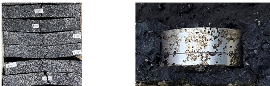
**Figure 8.** Specimen failure after the three-point bending test.
