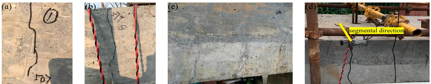
**Figure 7.** Development of cracks at the beginning of the test: (a) the first crack when the load was increased to 507 kN; (b) the crack when loaded to 579 kN; (c) cracks in midspan tensile zone when the load reached 650 kN; and (d) cracks in bottom plate developing along segments when loaded to 650 kN.
