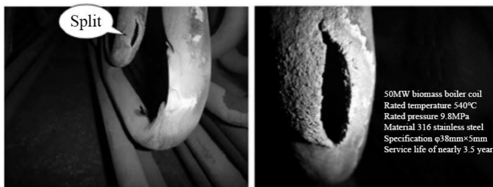
Figure 18. Rupture of coil in actual working condition.
