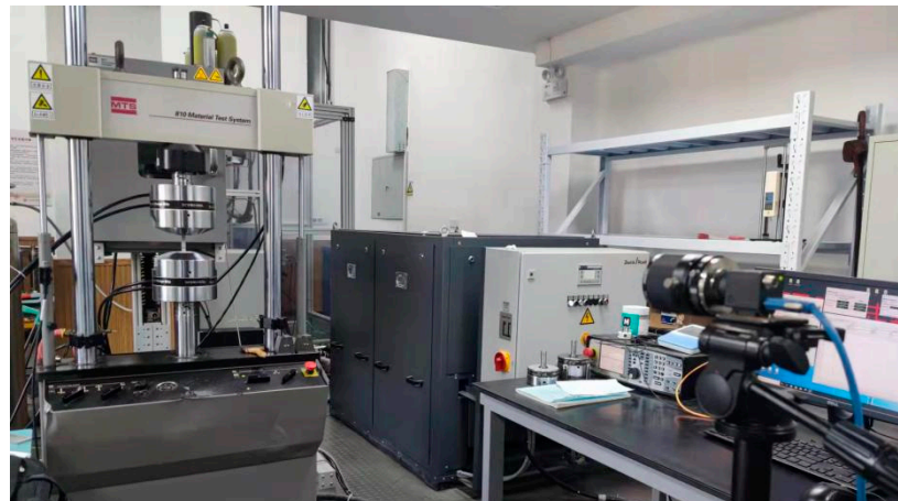
Figure 10. Uniaxial tensile test of specimens.
