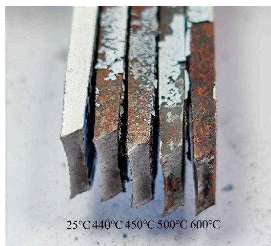
Figure 13. Fracture diagram of tensile specimen.
