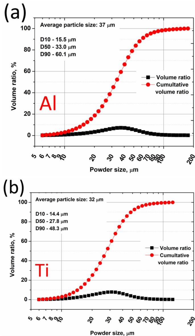
Figure 2. Al (a) and Ti (b) feedstock powder particle size distribution.
