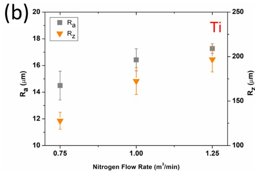
Figure 7. Surface roughness of Al (a) and Ti (b) coatings.
