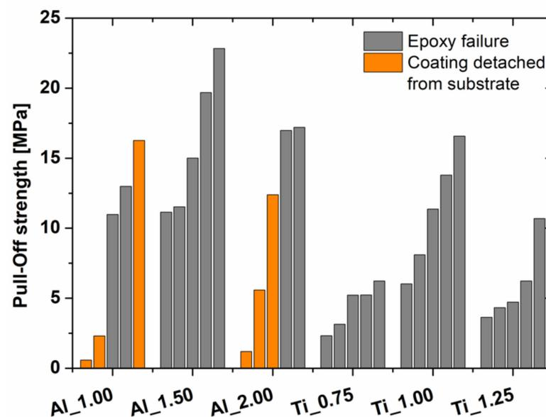
Figure 10. Pull-off strength of Al and Ti coatings.
