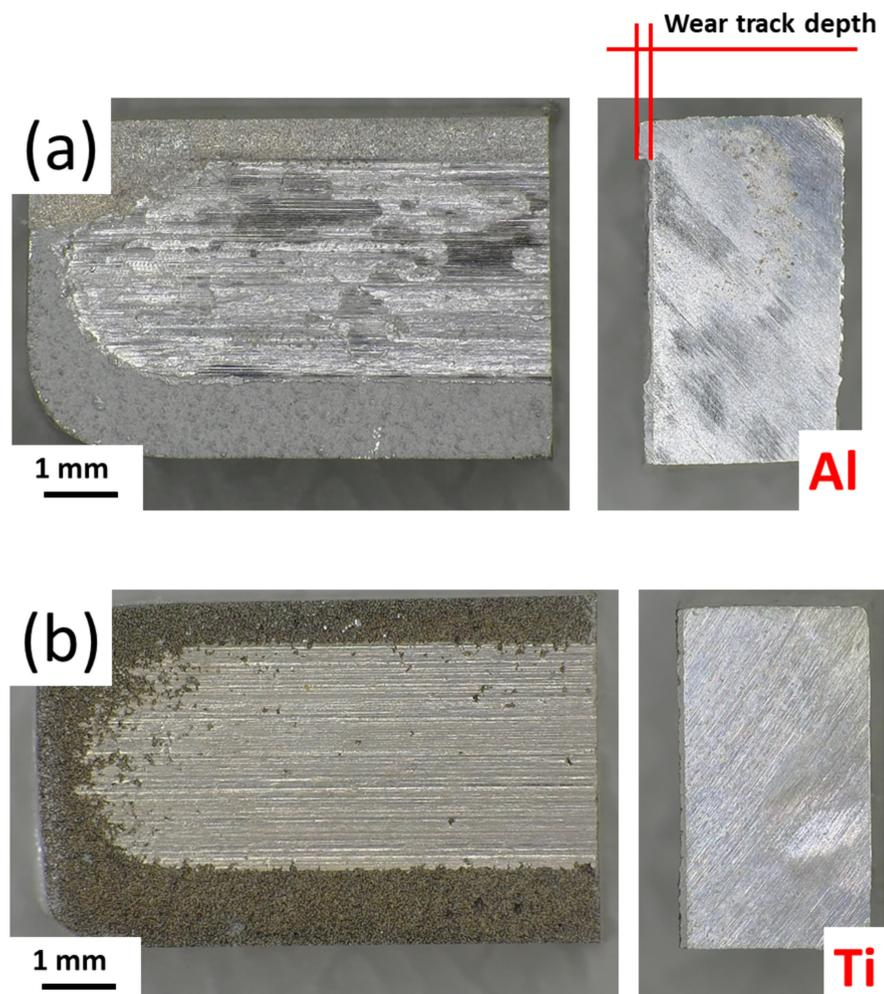
Figure 12. Top and cross-sectional view of Al<sub>1.5</sub> (a) and Ti<sub>1.0</sub> (b) coatings after pin on plate wear test.
