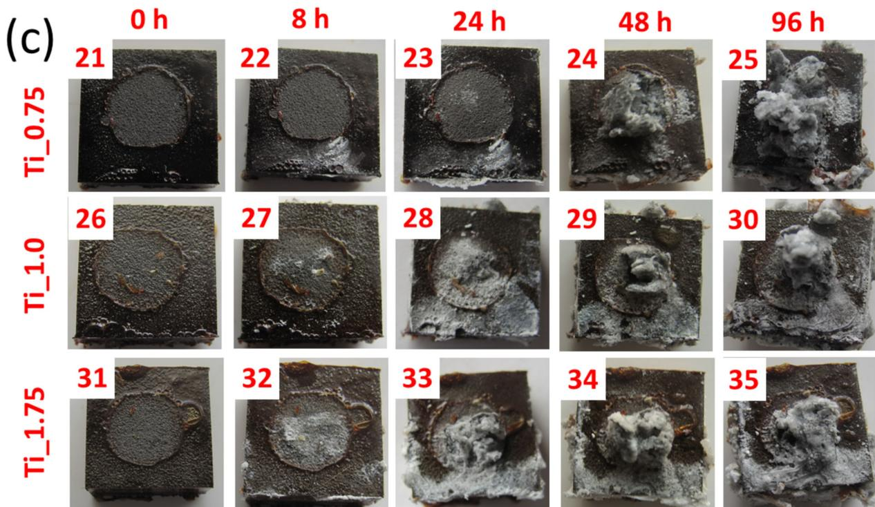
**Figure 9.** Surface observations at 0, 8, 24, 48, and 96 h of salt spray corrosion test for AZ91E substrate plate (a), WS Al (b) and Ti (c) coatings.
