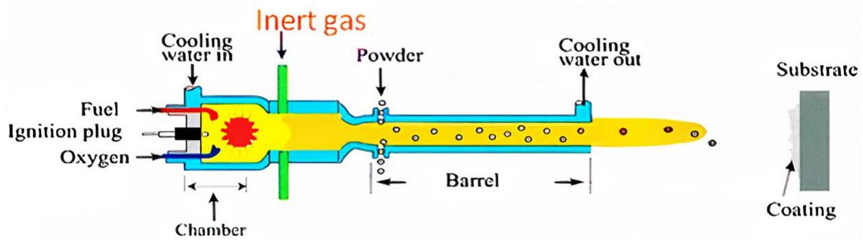
**Figure 3.** Schematic of the WS gun [29]. Reproduced with permission from Kuroda, S. et al., Journal of Thermal Spray Technology; published by Springer Nature, 2011.
