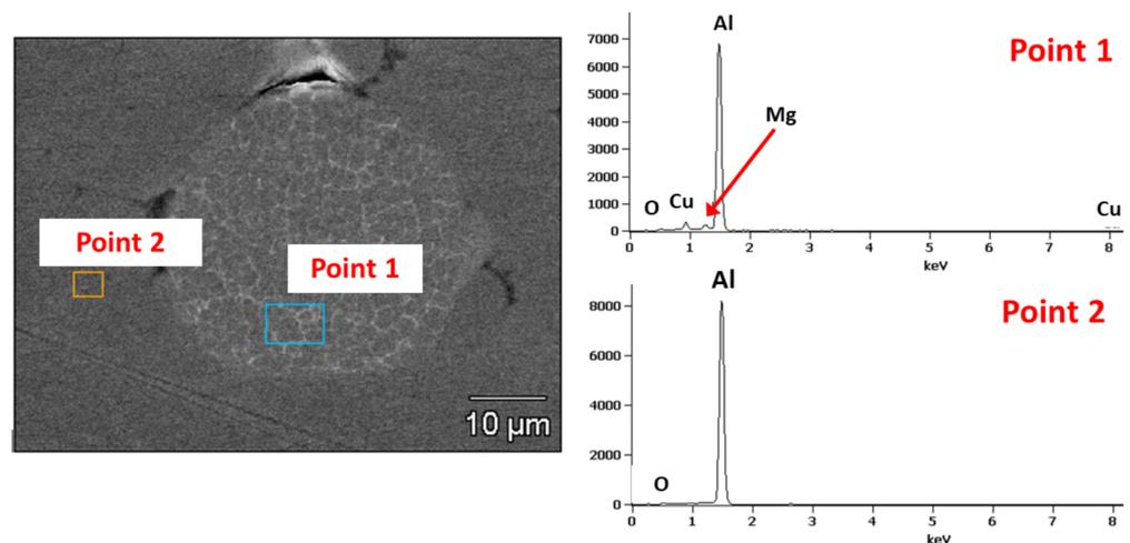
**Figure 5.** EDS analysis of contamination particles in Al coatings.
