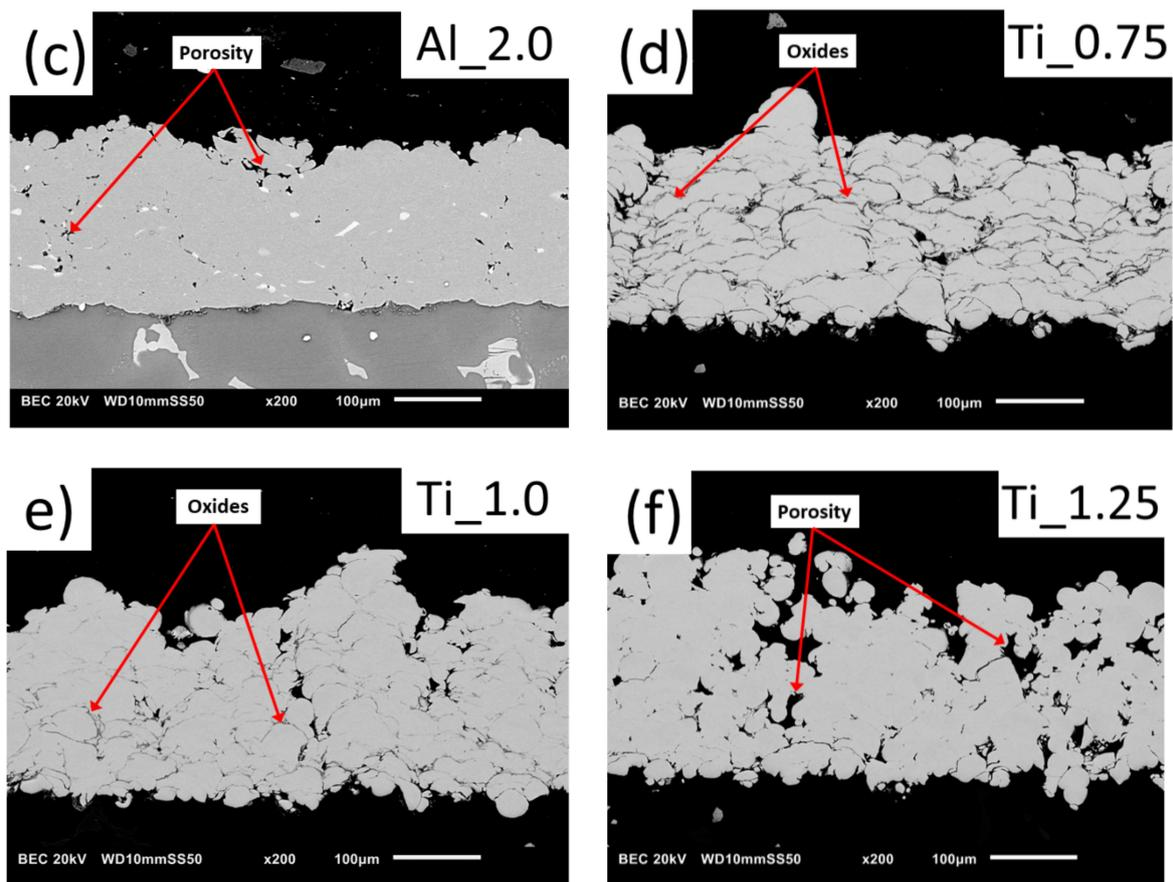
**Figure 4.** SEM images of cross-sections of WS coatings: (a) Al\_1.0, (b) Al\_1.5, (c) Al\_2.0, (d) Ti\_0.75, (e) Ti\_1.0, and (f) Ti\_1.25.
