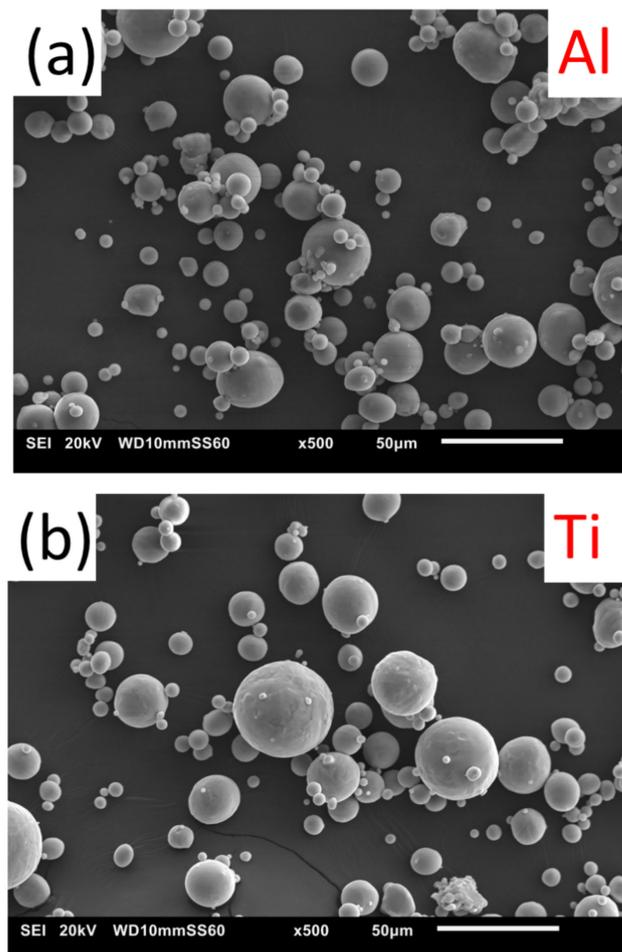
Figure 1. SEM images of Al (a) and Ti (b) feedstock powder used to produce WS coatings.
