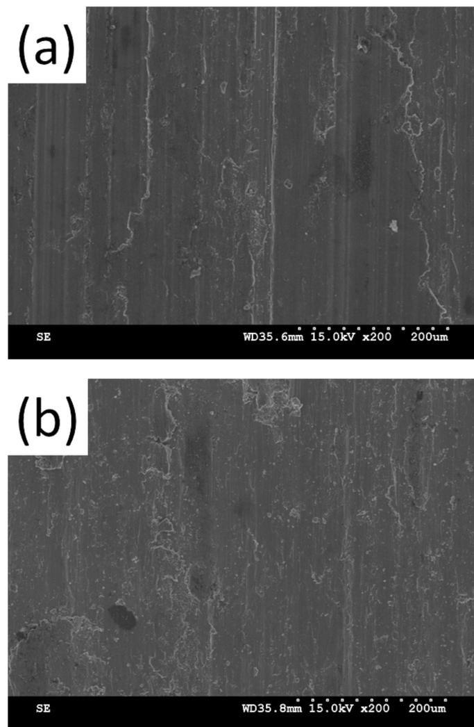
Figure 13. SEM images of wear track for Al (a) and Ti (b) coatings.
