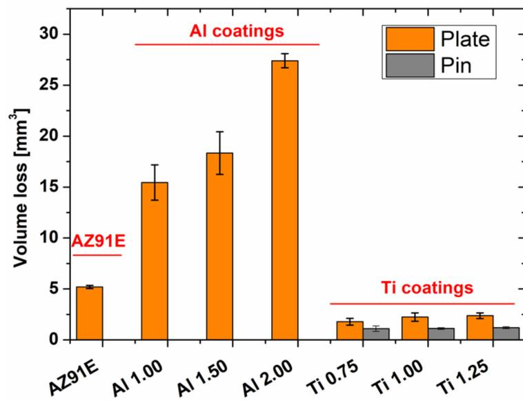
Figure 11. Volume loss of Al and Ti coatings, AZ91E substrate plate and pin material.
