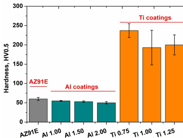
Figure 8. Hardness of Al, Ti coatings and AZ91E substrate plate.
