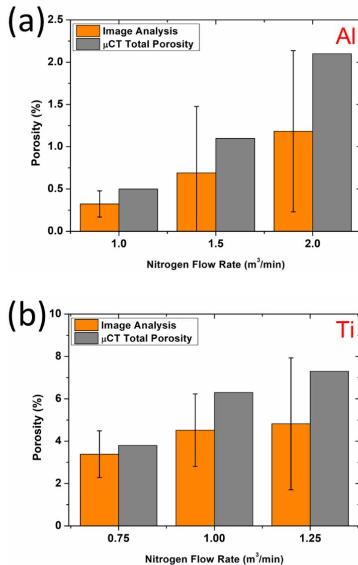
Figure 6. Porosity of Al (a) and Ti (b) coatings.
