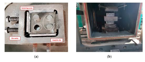
**Figure 3.** Graphite die and installation: (a) Graphite die; (b) Die Installation.
