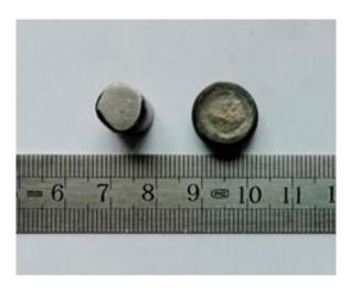
Figure 5. Samples after canning and isothermal compression.
