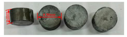
Figure 4. Sintered Zr-6Al-0.1B alloy workpieces.
