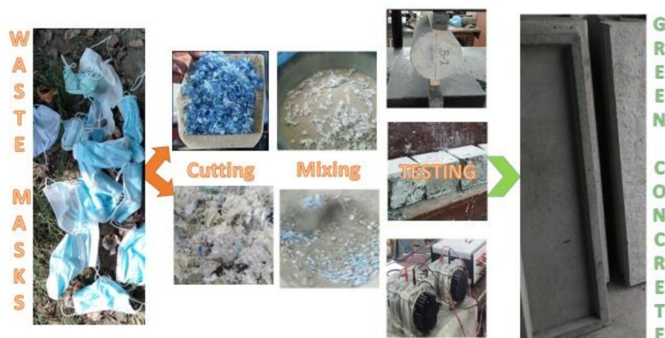
**Figure 1.** Methodology to use waste masks in concrete.
