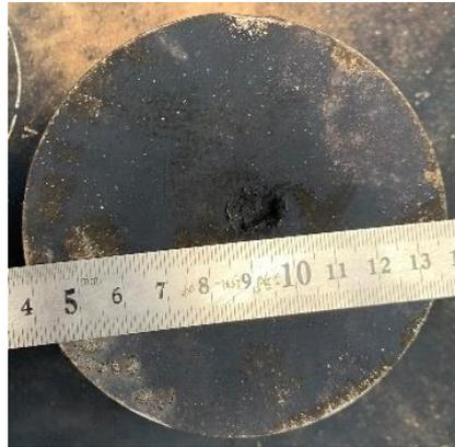
**Figure 20.** Experimental result of the steel plate impacted by the PTFE/Al reactive composite jet.
