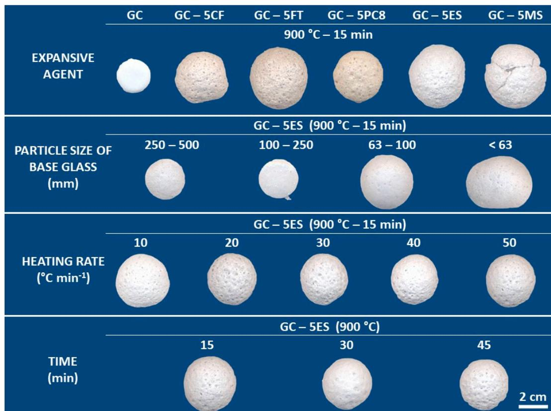
**Figure 3.** Appearance of the glass lightweight aggregates after the expansion tests performed with different processing parameters on pressing pellets.
