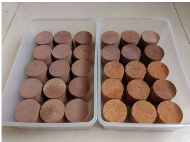
**Figure 4.** Specimens for the unconfined compression test.
