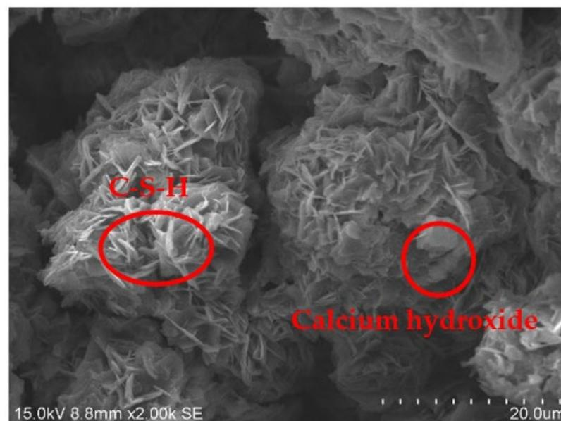
Figure 15. Image of the hydration products of the  $\text{A}_1\text{BC}_2$  Combination (2).
