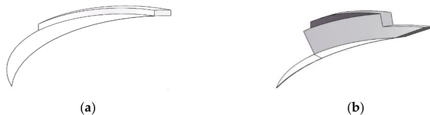
**Figure 15.** Chip simulation. (a) Chips formed by the flat-bottomed reverse edge cutting cutter; (b) chips formed by the gradual-removal reverse edge cutting cutter.
