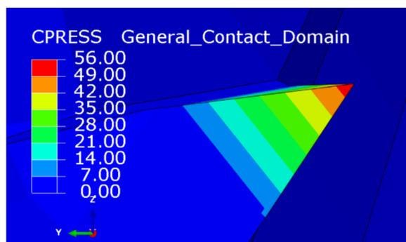
Figure 10. The cutting force distribution of the flat-bottomed reverse edge.
