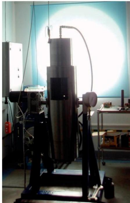
**Figure 1.** Hydrostatic extrusion press.
