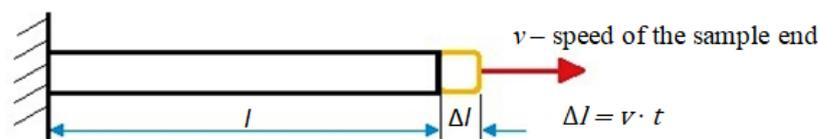
**Figure 11.** Sample deformation over time [25].
