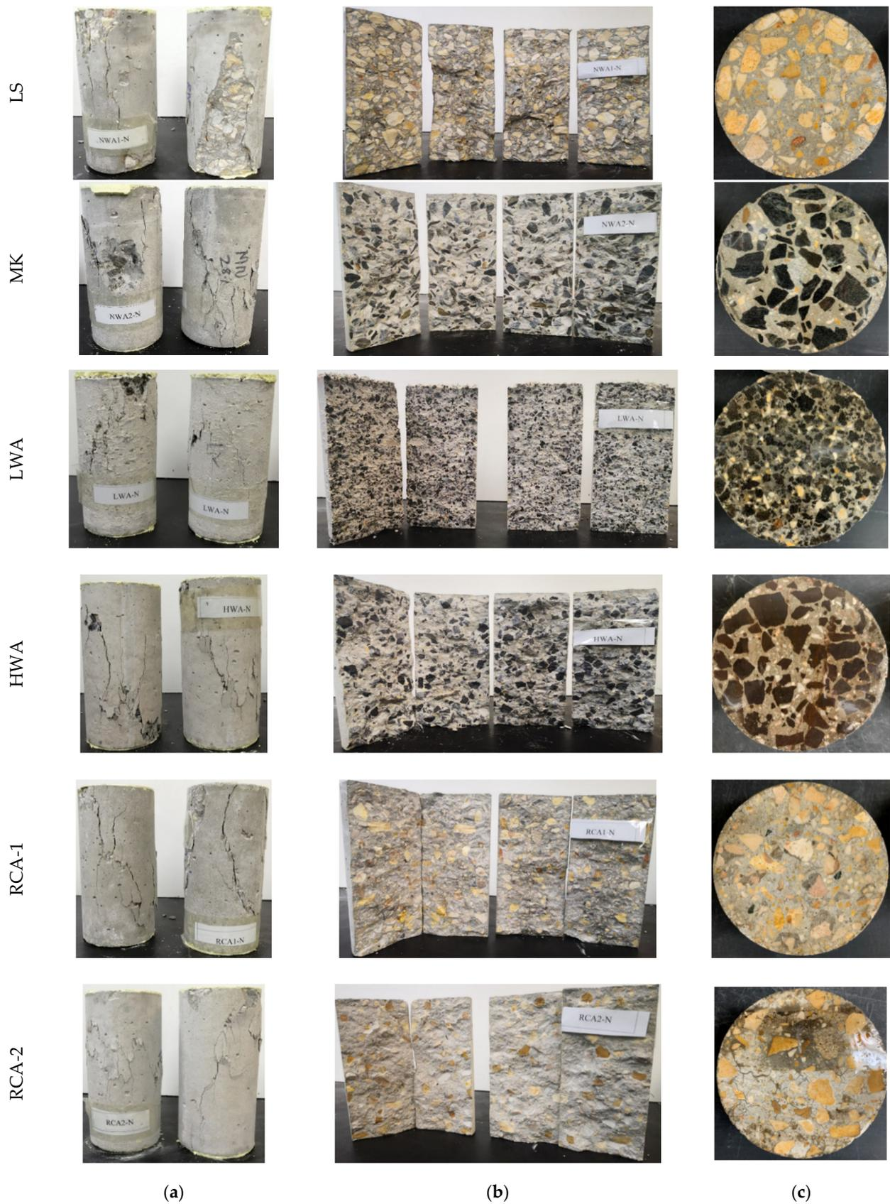
**Figure 4.** Illustrative photographs of Mix 2: (a,b) compression and splitting tension failure; and (c) cross section.
