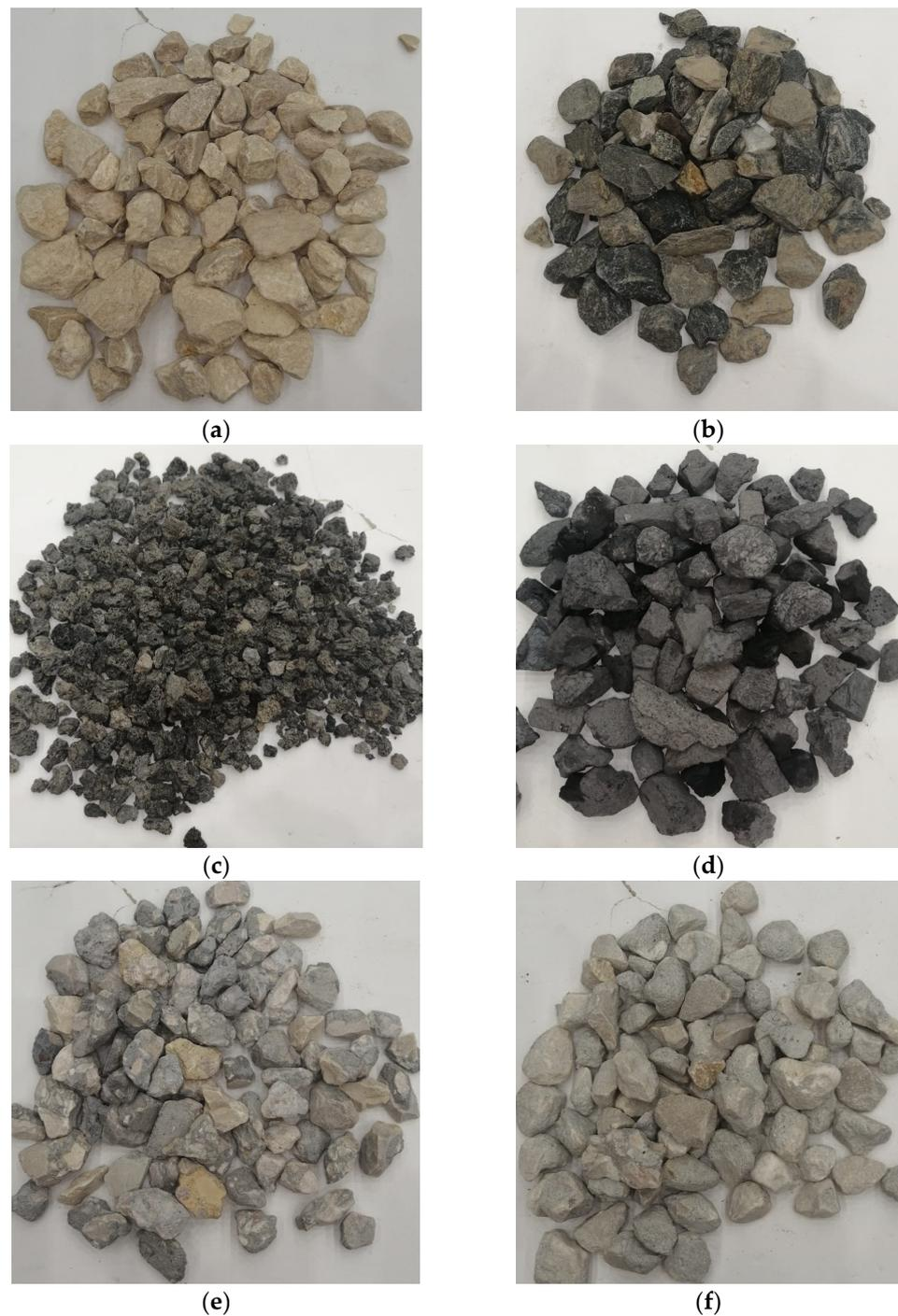
**Figure 1.** Illustrative pictures of various coarse aggregate types investigated in this study: (a) limestone-based normal weight aggregate (LS), (b) natural quartzite-based normal weight aggregate (MK), (c) volcanic scoria-based LWA, (d) by-product industrial waste steel slag-based HWA, (e) good quality recycled concrete-based normal weight aggregate (RCA-1), and (f) poor quality recycled concrete-based normal weight aggregate (RCA-2).
