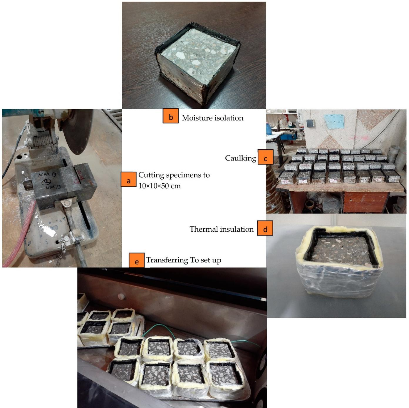
Figure 5. Preparation stages of freeze-thaw test samples.
