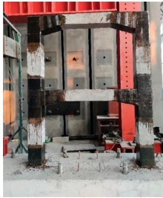
(b) Strengthening with CFRP
