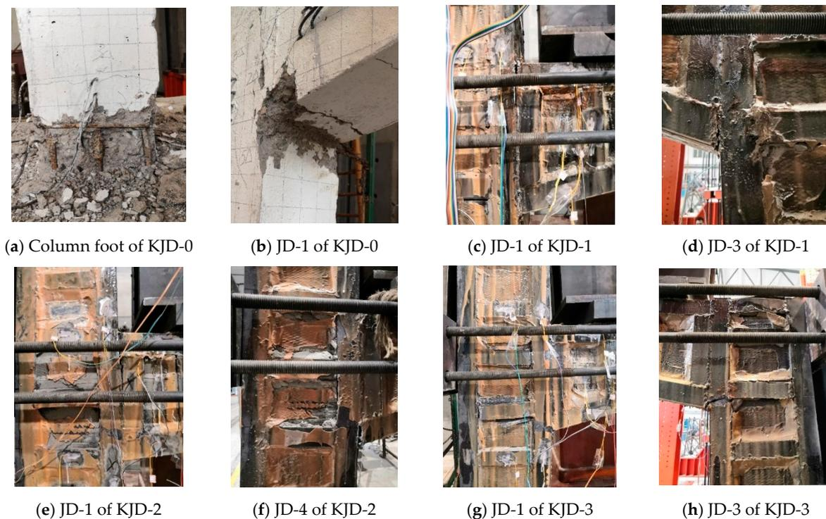
**Figure 8.** Typical failure phenomenon of specimens.
