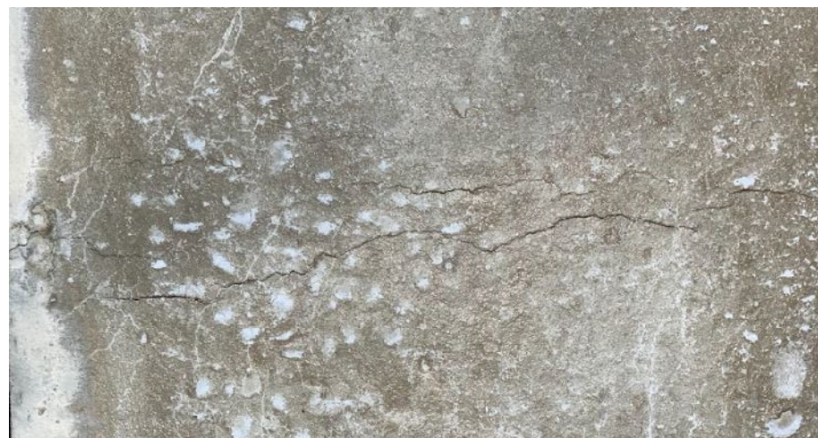
Figure 11. Typical crack pattern in plain concrete (PC) specimens of high temperature examined at 24 h.
