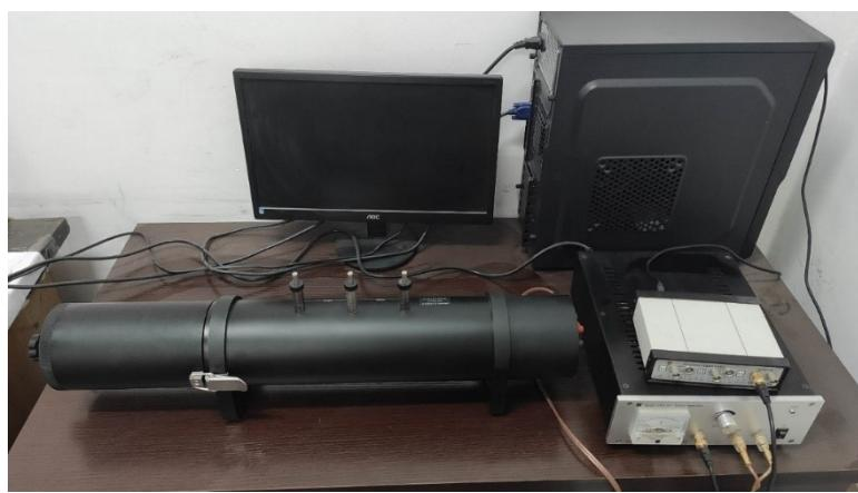
**Figure 9.** Sound absorption coefficient test equipment.
