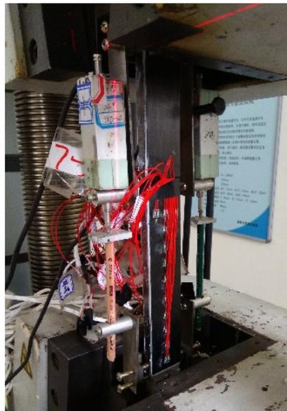
Figure 3. Test setup and instrumentation for the double-lap joint tensile tests.
