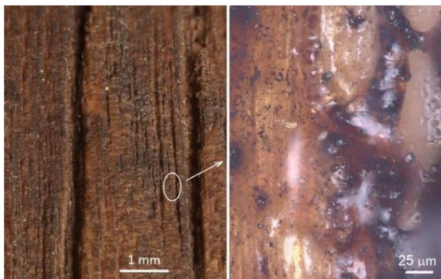
**Figure 7.** Surface of oak wood engraved with a CO<sub>2</sub> laser at laser power of 16 % and raster density of 30 mm<sup>-1</sup>. **Left:** radial surface with obvious trenches in early wood. **Right:** melt layer topping the engraved surface—detail.
