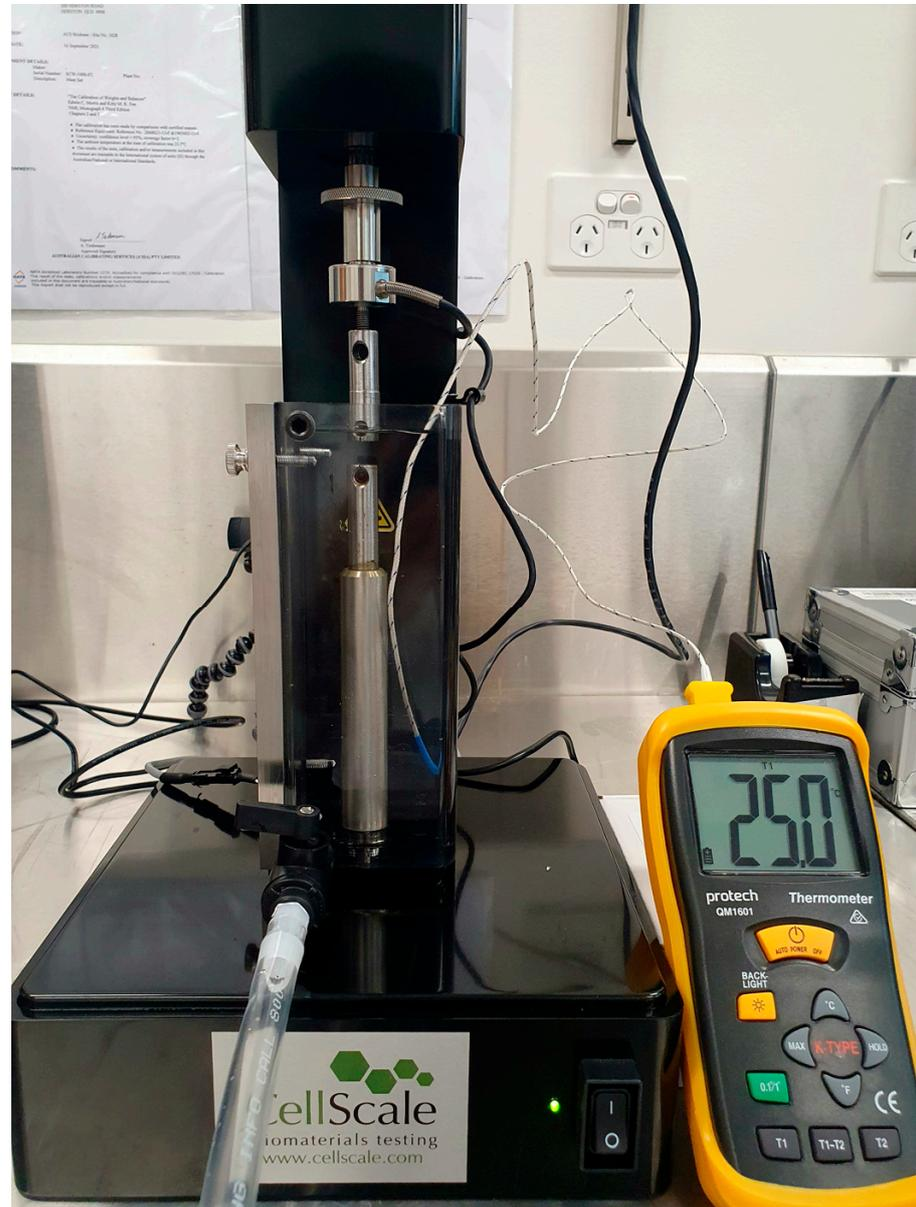
**Figure 5.** Photograph of UniVert microtensile test setup used.
