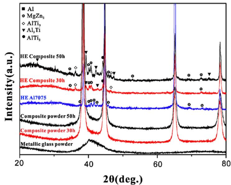
**Figure 16.** XRD patterns of the  $\text{Ti}_{52}\text{Cu}_{20}\text{Ni}_{17}\text{Al}_{11}$  metallic glass, Al 7075 + 8 vol.%  $\text{Ti}_{52}\text{Cu}_{20}\text{Ni}_{17}\text{Al}_{11}$  mixtures, hot-extruded matrix alloy, and composites obtained from the Al 7075 + 8 vol.%  $\text{Ti}_{52}\text{Cu}_{20}\text{Ni}_{17}\text{Al}_{11}$  mixtures milled for 30 h and 50 h. Reprinted from [67], Copyright (2018), with permission from Elsevier.
