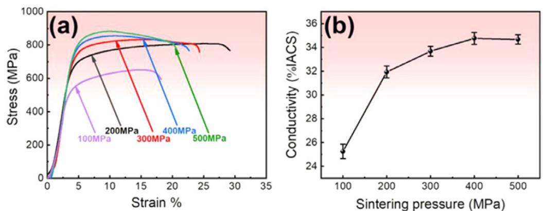
**Figure 19.** (a) Engineering stress–strain curves of composites obtained via SPS of CuCrZr alloy + 24 wt.% Cu<sub>50</sub>Zr<sub>43</sub>Al<sub>7</sub> metallic glass mixtures at 693 K and different pressures; (b) variation in the electrical conductivity of the composites with the sintering pressure. Reprinted from [88], Copyright (2022), with permission from Elsevier.
