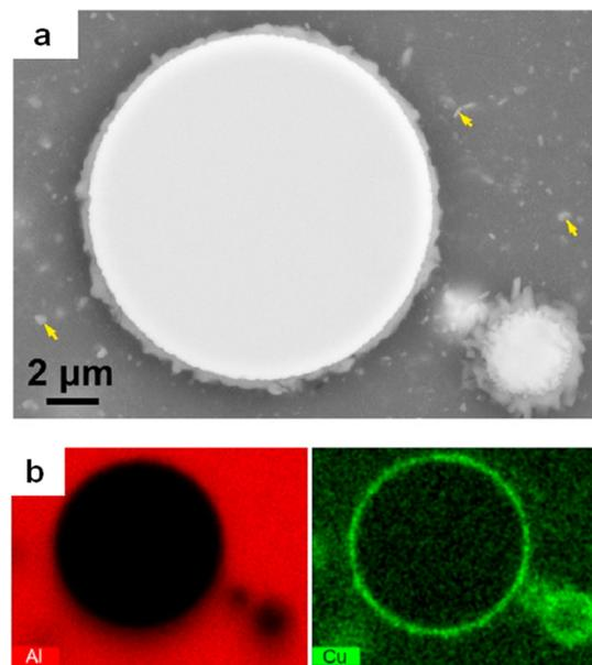
**Figure 14.** (a) A micrograph showing a particle of the Fe<sub>43.2</sub>Co<sub>28.8</sub>B<sub>19.2</sub>Si<sub>4.8</sub>Nb<sub>4</sub> metallic glass in the matrix of Al 2024 alloy. The composite was heat-treated. (b) Maps of Al and Cu; the map of Cu shows its concentration at the interface. Reprinted from [78], Copyright (2020), with permission from Elsevier.
