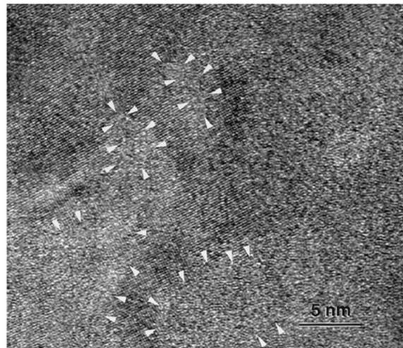
**Figure 2.** High-resolution transmission electron microscopy image of a rapidly solidified Al-4V-2Fe alloy. Amorphous regions surrounded by the interconnected  $\alpha$ -Al phase are arrowed. Reprinted from [38], Copyright (1998), with permission from Elsevier.
