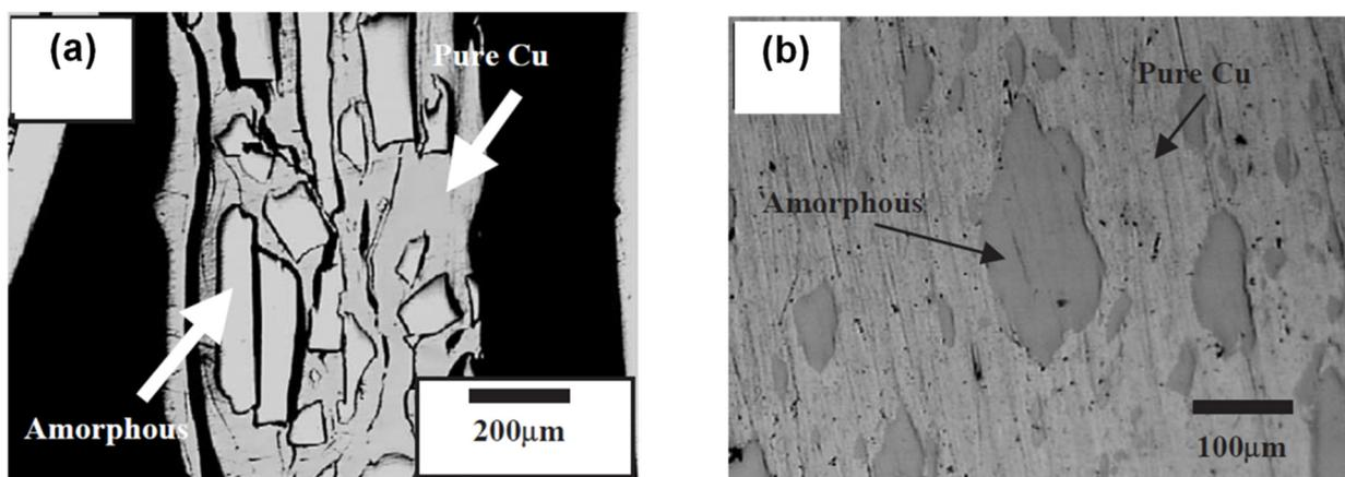
**Figure 4.** Microstructure of Cu + Ni-Zr-Ti-Si-Sn metallic glass composites obtained via (a) cold rolling and folding of Cu foils with Ni-Zr-Ti-Si-Sn metallic glass ribbons, (b) warm rolling of cold-rolled composites sealed in a Cu tube. Reprinted from [36], Copyright (2004), with permission from Elsevier.
