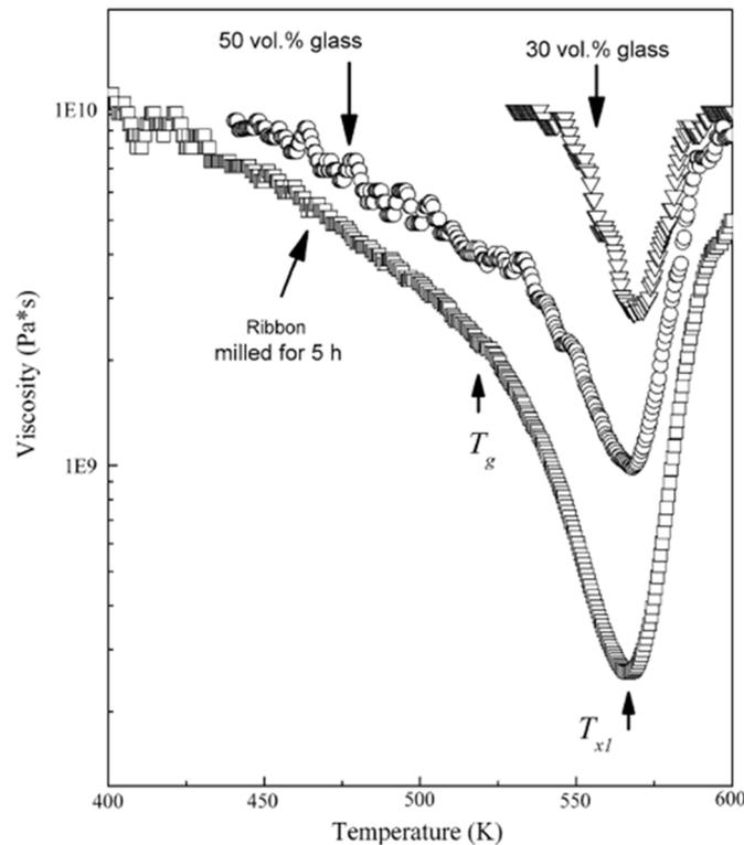
**Figure 6.** Temperature dependence (heating rate  $10\text{ K min}^{-1}$ ) of the viscosity of the supercooled liquid for the single-phase  $Al_{85}Y_8Ni_5Co_2$  glassy ribbon (mechanically milled) and for the Al matrix composites with 50 vol.% and 30 vol.% glass reinforcement. Reprinted from [45], Copyright (2008), with permission from Springer Nature.
