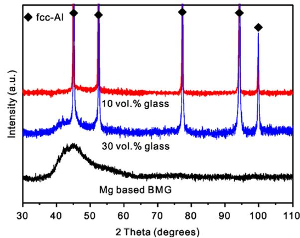
**Figure 8.** X-ray diffraction (XRD) patterns of the  $Mg_{65}Cu_{20}Zn_5Y_{10}$  glass and Al +  $Mg_{65}Cu_{20}Zn_5Y_{10}$  composites. Reprinted from [58], Copyright (2014), with permission from Elsevier.
