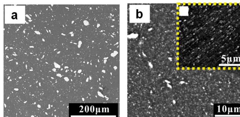
**Figure 15.** Microstructure of the hot-extruded composites obtained from Al 7075 + 8 vol.%  $\text{Ti}_{52}\text{Cu}_{20}\text{Ni}_{17}\text{Al}_{11}$  mixtures milled for 10 h (a) and 50 h (b). Reprinted from [67], Copyright (2018), with permission from Elsevier.
