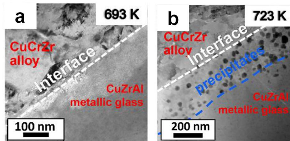
**Figure 12.** Transmission electron microscopy images of the interface in composites obtained via spark plasma sintering of CuCrZr alloy + 30 wt.% Cu<sub>50</sub>Zr<sub>43</sub>Al<sub>7</sub> metallic glass mixtures at 500 MPa at different temperatures: (a) 693 K and (b) 723 K. Reprinted from [88], Copyright (2022), with permission from Elsevier.
