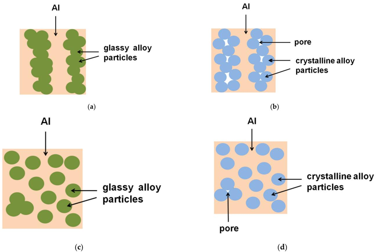
**Figure 11.** Schematic of the microstructures of aluminum matrix composites formed using a glassy (a,c) or a crystalline (b,d) alloy reinforcement. Reprinted from [82]. This article is an open access article distributed under the terms and conditions of the Creative Commons Attribution (CC BY) license (<https://creativecommons.org/licenses/by/4.0/>).
