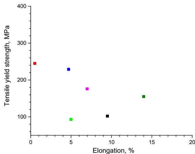
**Figure 18.** Tensile yield strength–elongation data for Al and Al alloy matrix composites: ■ Al + Ni<sub>60</sub>Nb<sub>40</sub> [55]; ■ Al-Zn-Ca + Co<sub>48</sub>Cr<sub>15</sub>Mo<sub>14</sub>C<sub>15</sub>B<sub>6</sub>Tm<sub>2</sub> [73]; ■, ■ Al 2024 + Fe<sub>49.9</sub>Co<sub>35.1</sub>Nb<sub>7.7</sub>B<sub>4.5</sub>Si<sub>2.8</sub> [57]; ■ Al + Al<sub>84</sub>Gd<sub>6</sub>Ni<sub>7</sub>Co<sub>3</sub> [56]; ■ Al + Zr<sub>48</sub>Cu<sub>36</sub>Ag<sub>8</sub>Al<sub>8</sub> [69].
