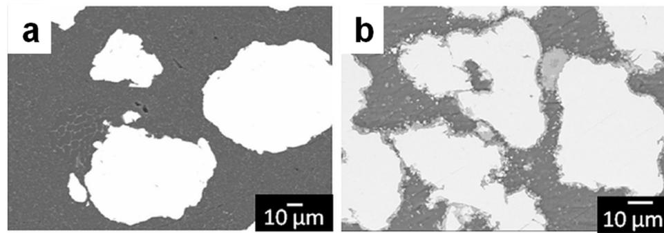
**Figure 13.** Microstructure of composites obtained from Al 2024 + 40 vol.% Ni<sub>60</sub>Nb<sub>40</sub> mixtures: (a) as-hot-pressed state and (b) heat-treated state. Reprinted from [71], Copyright (2019), with permission from Elsevier.
