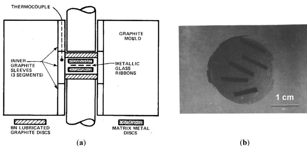
**Figure 1.** Schematic of the assembly for hot pressing of the ribbons with metal discs (a) and a radiograph of the hot-pressed sample (b). Reprinted from [29], Copyright (1982), with permission from Springer Nature: Chapman and Hall, Ltd.
