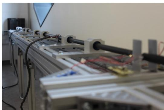
**Figure 3.** Developed Kolsky compression bar for elastomer testing.
