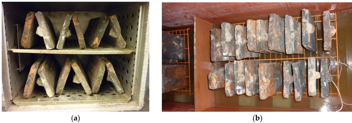
Figure 5. Absorption test: (a) drying of tiles to constant weight at a temperature of 110\text{ }^{\circ}\text{C} \pm 5\text{ }^{\circ}\text{C} ; (b) roof tiles in a chamber with 100% humidity.
