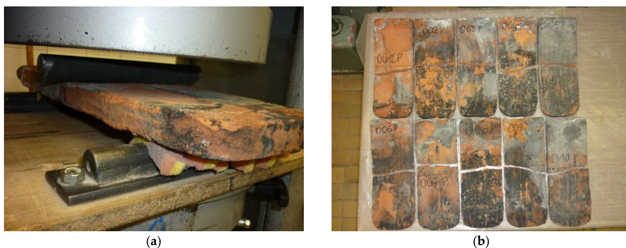
Figure 11. Flexural load capacity test: (a) tile in the testing machine during flexural capacity tests; (b) tiles (Nos. 001–010) after flexural strength tests.
