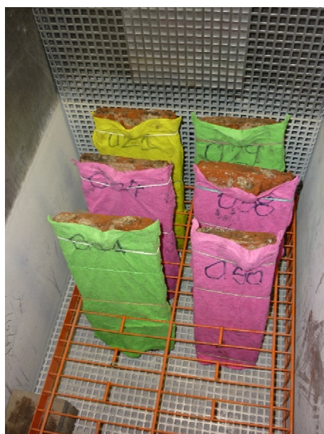
Figure 7. Roof tiles in a climate chamber.
