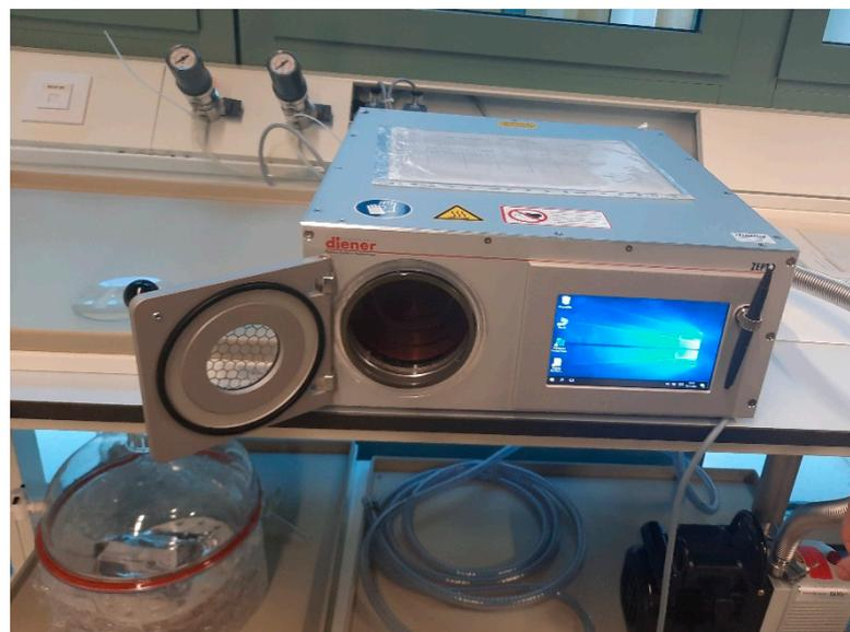
**Figure 5.** Low-pressure plasma apparatus used with argon and with polymerization treatment.
