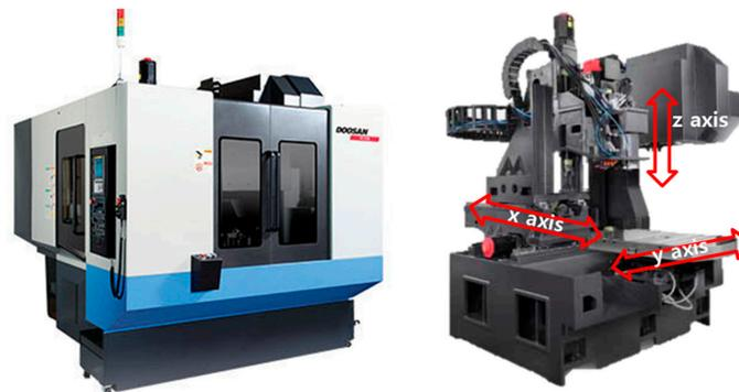
Figure 1. Three-axis machining center.
