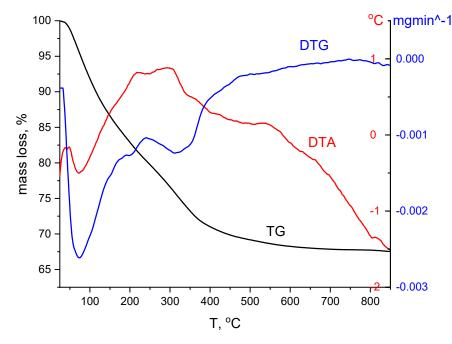
Figure 1. Thermogravimetric analysis for MgFe<sub>2</sub>O<sub>4</sub> material.
