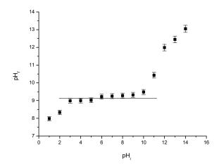
Figure 4.  $pH_{pZc}$  for MgFe<sub>2</sub>O<sub>4</sub> material treated at 260 °C.
