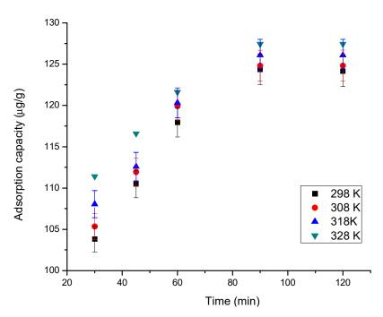
Figure 6. Contact time and temperature effect.
