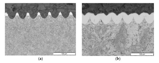
**Figure 3.** (a) LOM cross-section image of the laser-textured sample before hardening. (b) The image shows a cross-section of the sample after the TRD CrC hardening process. The sample in the images has a depth of craters  $\sim$ 30 µm and a spot-to-spot spacing  $\sim$ 50 µm.
