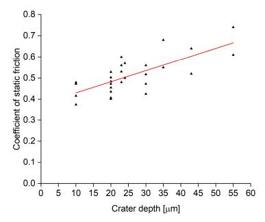
**Figure 11.** Static friction coefficient as a function of crater depth. The results presented here were obtained with both the 20 W and 200 W lasers. Results include various spot-to-spot spacings. The results for the same crater depth are for a range of different spot-to-spot spacings, hence the spread of coefficient of friction values.
