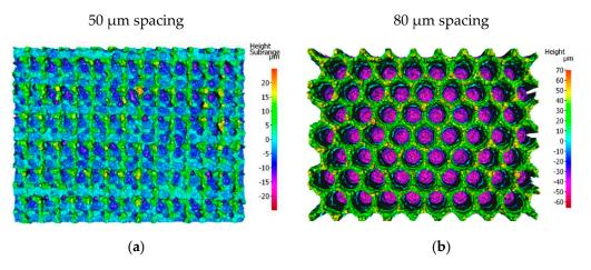
**Figure 7.** Figure shows the topography of laser structures with (**a**) 50  $\mu$ m and (**b**) 80  $\mu$ m spot-to-spot spacing.
