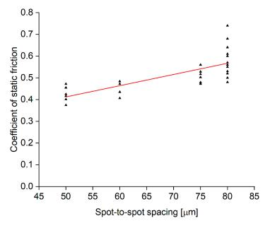
**Figure 12.** Static friction coefficient as a function of spot-to-spot spacing. The results presented here were obtained with both the 20 W and 200 W lasers. The results for the same spot-to-spot spacing are for a range of different crater depths, hence the spread of coefficient of friction values.
