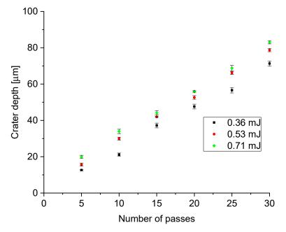
**Figure 5.** Crater depth as a function of the number of laser passes for three different pulse energies. Results presented for the 20 W laser.
