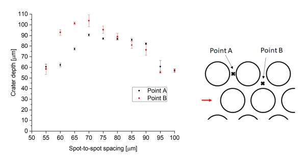
**Figure 6.** Height of the two key points between adjacent craters. The maximum pulse energy used was 0.71 mJ.
