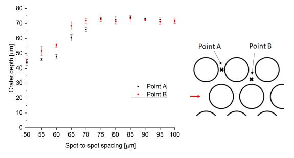
**Figure 9.** Height of the two key points between adjacent craters. The pulse energy used was 1.46 mJ, with the 200 W SPI laser.
