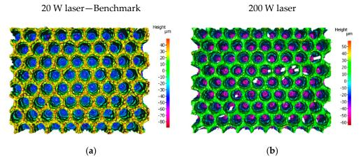
**Figure 10.** Comparison of the surface topographies for processing with 20 W laser (**a**) and 200 W laser (**b**).
