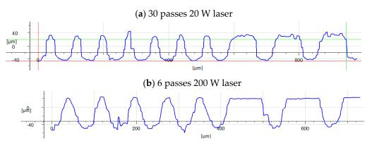
**Figure 8.** Cross-section surface profile of topographies achieved by the 20 W laser (**a**) and 200 W laser (**b**).
