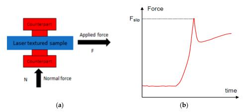
**Figure 4.** (a) Schematic of the static friction coefficient testing setup. (b) Typical plot of force as a function of time during the test.
