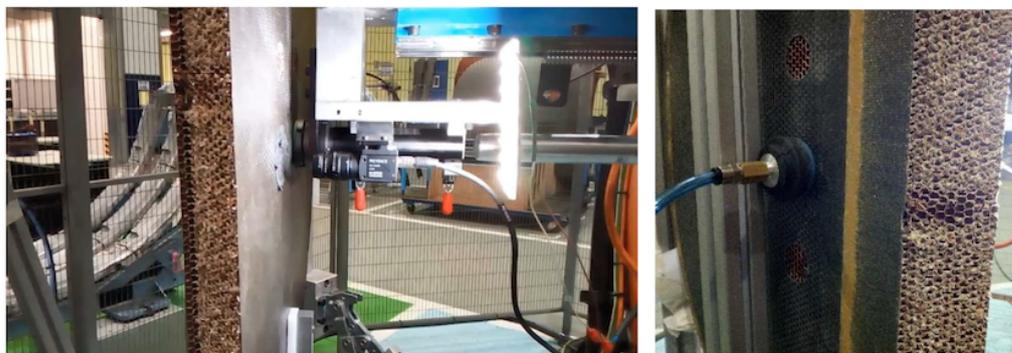
**Figure 9.** Test of the vacuum-assisted multi cell injection system. **Left:** The end-effector is located at one side of the panel by the robot arm. The optical camera and light-panel help the operation. **Right:** A vacuum nozzle is located at the opposite side of the panel to assist the resin injection.
