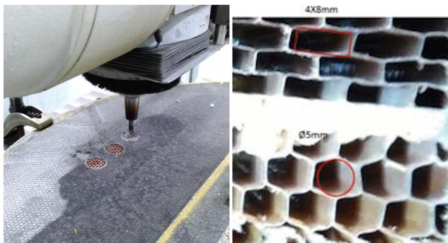
**Figure 4.** LEFT: Conventional milling operation to remove the CFRP skin of a sandwich panel made with the same cutting tool mounted in the designed end-effector. RIGHT: Detail of the honeycomb panel made of NOMEX, which combines two cell shapes and sizes under the skin.
