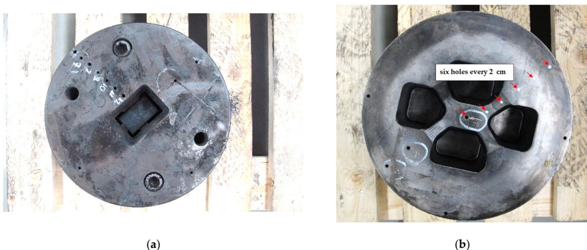
**Figure 13.** Dies with marked places of thermocouples that measure the achieved temperature during annealing at 460 °C. (a) first example of die; (b) second example of die.
