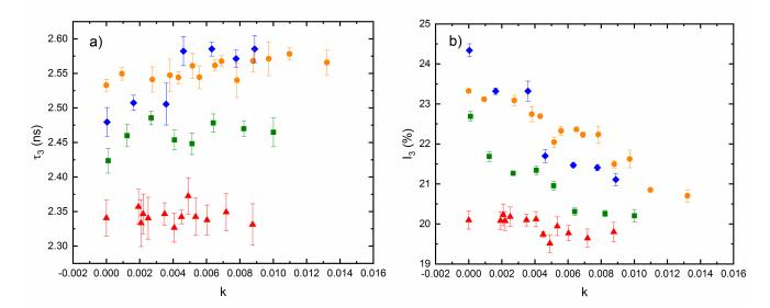
**Figure 10.** The o-Ps lifetime (**a**) and their relative intensity  $I_3$  (**b**) as a function of water content expressed by *k* for the investigated samples. AESO/VDM squares, AESO/VDM/DMPA triangles, ELO/PI dots, and ELO/10RD1/PI diamonds.
