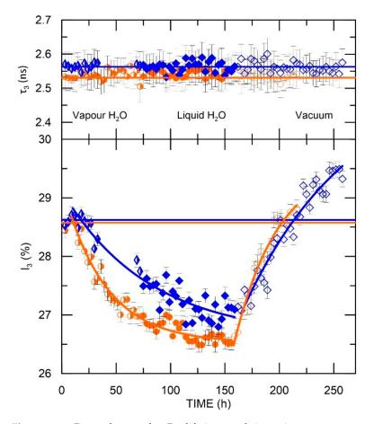
**Figure 7.** Dependence of o-Ps lifetime and intensity on water presence (ELO/PI—dots, ELO/10RD1/PI—diamonds); half-full points, full points, and empty points represents stage 1, 2, and 3 of measurement regime, respectively.
