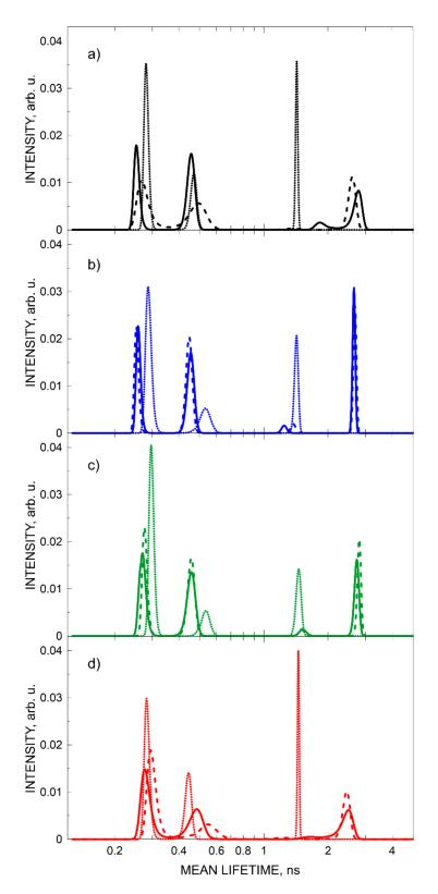
**Figure 3.** Distribution of mean lifetimes in the PALS spectrum of samples (**a**) ELO/PI, (**b**) ELO/10RD1/PI, (**c**) AESO/VDM, and (**d**) AESO/VDM/DMPA obtained from MELT processing of the spectra. Virgin sample at 18 °C (solid line), sample at -150 °C (dotted line), and again at room temperature (dashed line).
