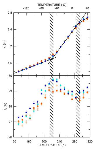
**Figure 4.** The o-Ps lifetime and intensity as a function of increasing (ELO/PI—orange dots, ELO/10RD1/PI—dark blue diamonds) and decreasing (ELO/PI—creamy dots, ELO/10RD1/PI—light blue diamonds) temperature.
