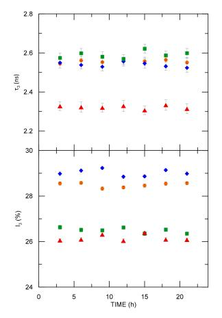
**Figure 2.** The o-Ps lifetime and intensity as a function of time for the four investigated samples at 18 °C; dots–ELO/PI, diamonds–ELO/10RD1/PI, squares–AESO/VDM, and triangles—AESO/VDM/DMPA.
