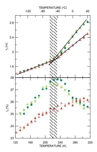
**Figure 5.** AESO/VDM, AESO/VDM/DMPA: the o-Ps lifetime and intensity as a function of increasing (AESO/VDM—dark green squares, AESO/VDM/DMPA—red triangles) and decreasing (AESO/VDM—light green squares, AESO/VDM/DMPA—pink triangles) temperature.
