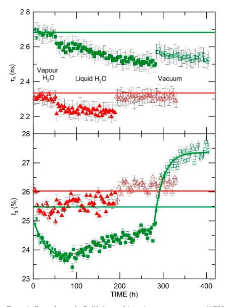
**Figure 8.** Dependence of o-Ps lifetime and intensity on water presence (AESO/VDM—squares, AESO/VDM/DMPA—triangles); half-full points, full points, and empty points represents the stage 1, 2, and 3 of measurement regime, respectively.
