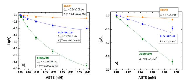
**Figure 12.** Calibration curves of chronoamperometric response (**a**) and analysis of linearity range and sensitivity (**b**) on the increasing concentrations of ABTS for the laccase bioelectrodes formed with different polymer matrixes. Conditions: working potential –100 mV vs. Ag/AgCl (3 M KCl), 50 mM acetate buffer, pH 4.5 at 23 °C and constant stirring.
