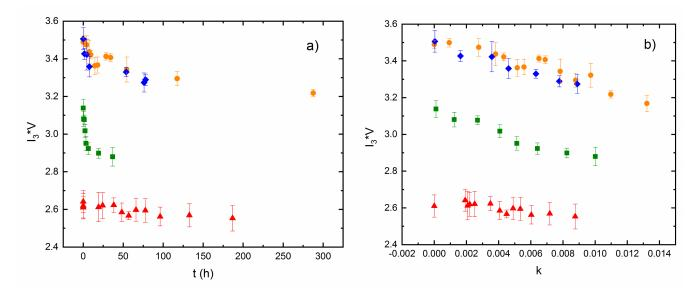
**Figure 11.** The reduced free volume fraction fv/C for the investigated samples as a function of time at swelling (reconstructed) (**a**) and as a function of water content expressed by k (**b**) AESO/VDM squares, AESO/VDM/DMPA triangles, ELO/PI dots, and ELO/10RD1/PI diamonds.
