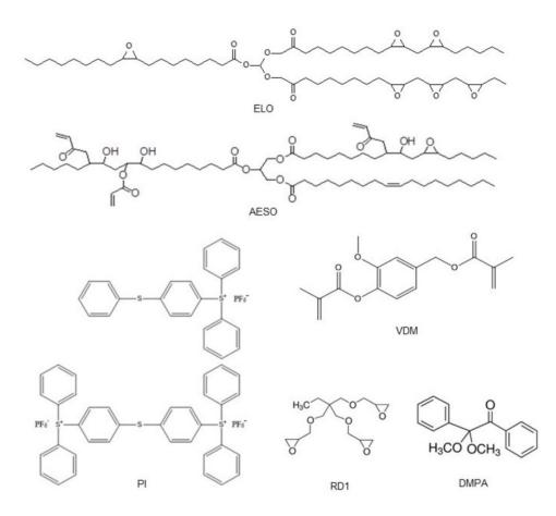
**Figure 1.** Chemical structures of epoxidized linseed oil (ELO), acrylated epoxidized soybean oil (AESO), trimethylolpropane triglycidyl ether (RD1), vanillin dimethacrylate (VDM), triarylsulfonium hexafluorophosphate salts (PI), and 2,2-dimethoxy-2-phenylacetophenone (DMPA).
