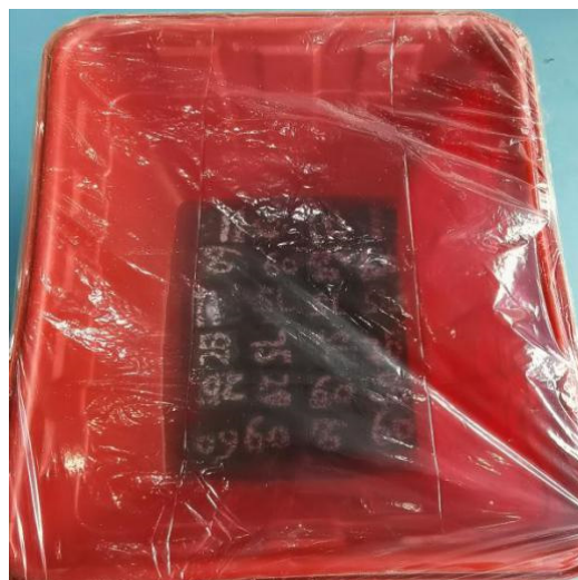
Figure 13. The acidic corrosion of the specimens.
