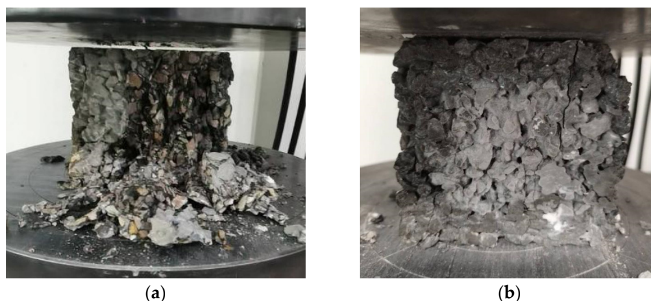
Figure 2. The failure patterns of (a) cubic specimens without basalt fiber and (b) cubic specimens with basalt fiber.
