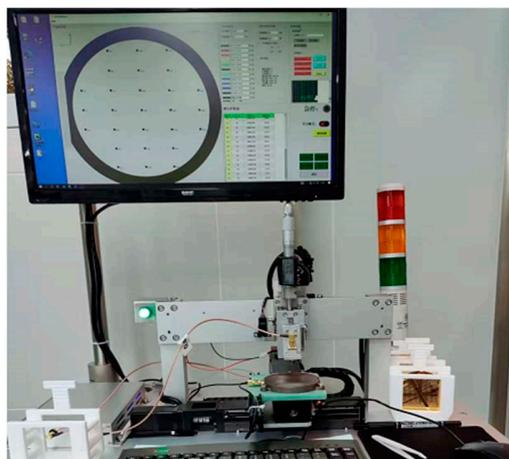
**Figure 2.** MT200 frequency tester.
