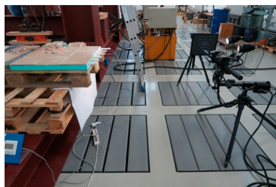
Figure 8. Digital image correlation system (DIC) for measuring LFS displacements.
