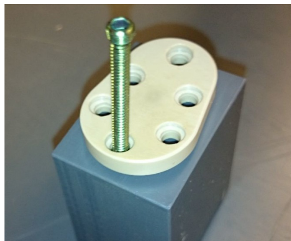
Figure 10. Fixing the test implant at the test block (represented is only one screw before insertion, the test implant was fixed with three screws).
