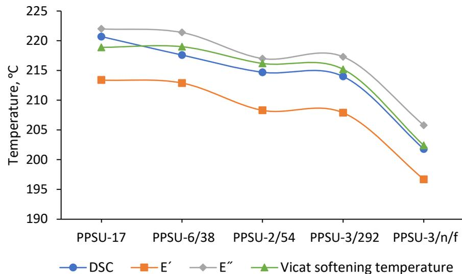
**Figure 3.** Tg and Vicat softening temperature curves of PPSU blends.
