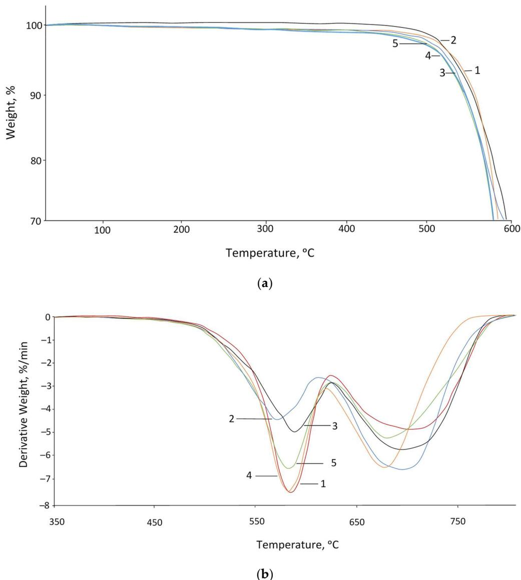
**Figure 5.** Mass loss curves (a) and derivatives of a mass loss curves (b) for PPSU blends: 1—PPSU-17; 2—PPSU-6/38; 3—PPSU-2/54; 4—PPSU-3/292; 5—PPSU-3/n/f.
