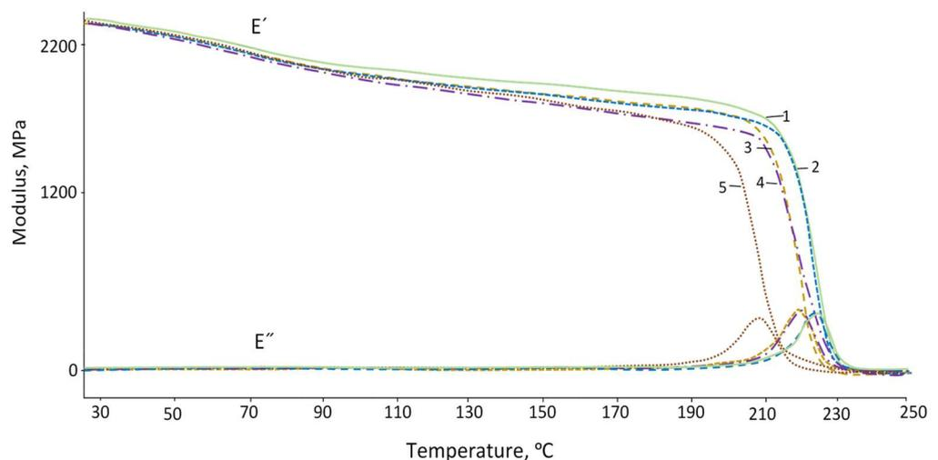
**Figure 2.** Storage modulus ( $E'$ ) and loss modulus ( $E''$ ) of PPSU blends: 1—PPSU-17; 2—PPSU-6/38; 3—PPSU-2/54; 4—PPSU-3/292; 5—PPSU-3/n/f.
