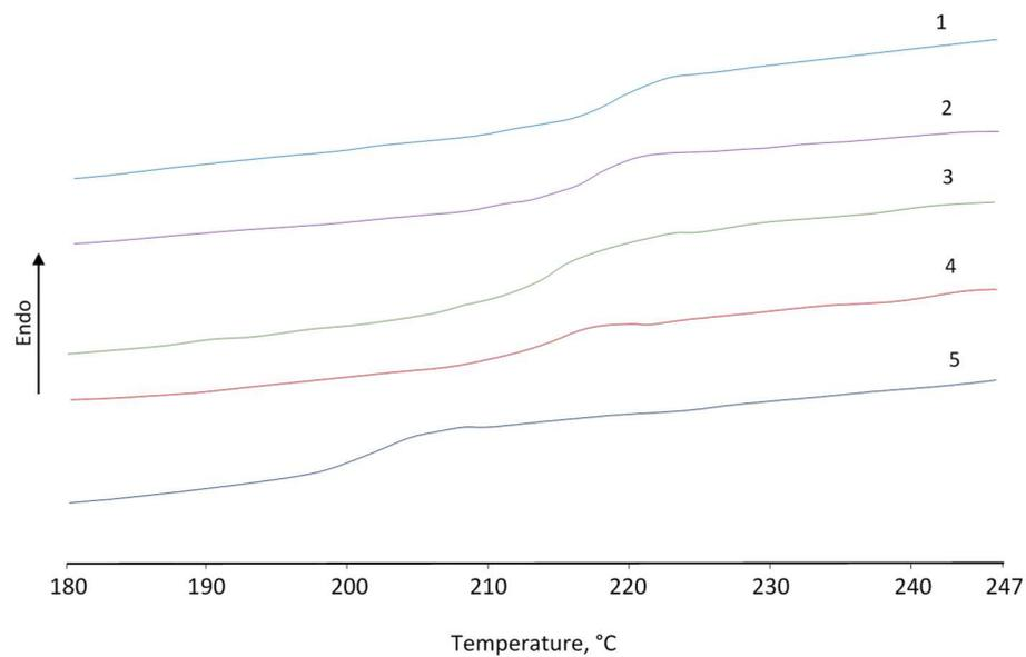
**Figure 1.** DSC curves of PPSU blends: 1—PPSU-17; 2—PPSU-6/38; 3—PPSU-2/54; 4—PPSU-3/292; 5—PPSU-3/n/f.
