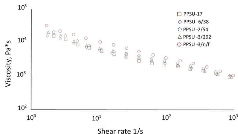
**Figure 4.** Flow curves of PPSU blends.
