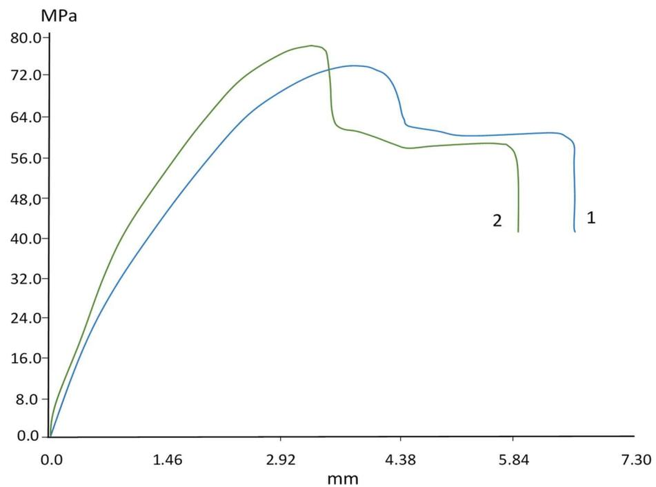
Figure 6. Stress-strain curves: 1—PPSU-17; 2—PPSU-3/n/f.
