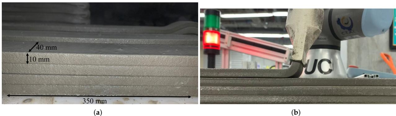
**Figure 6.** (a) 3D printed filaments for mechanical tests. (b) UHPC being printed.
