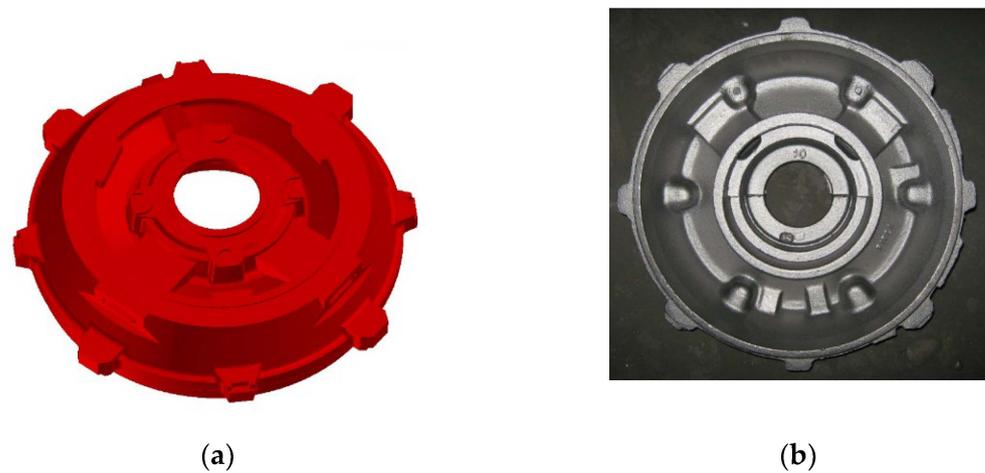
**Figure 5.** (a) Three-dimensional solid and (b) actual appearance of tested cast of electric motor shield.
