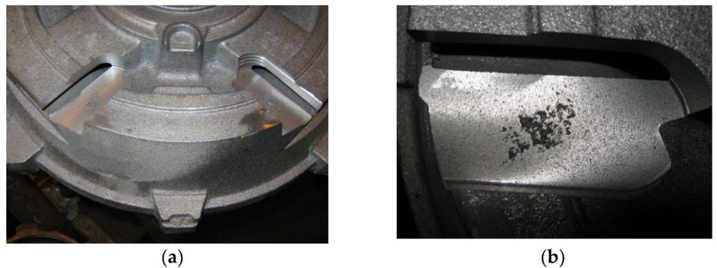
**Figure 6.** (a) Place of appearance of porosity in cast of motor shield and (b) appearance of defect.
