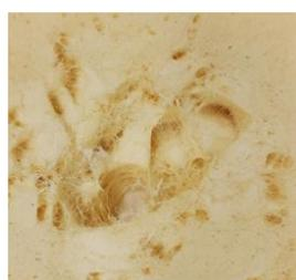
**Figure 9.** Disturbances in the cellular structure of the foam W22\_0.6.
