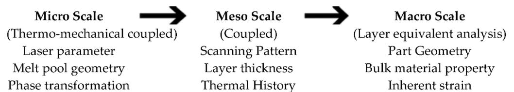
**Figure 1.** Multi-scale simulation approach in AM distortion analysis.
