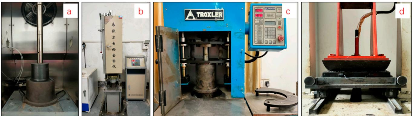
**Figure 2.** Test setup for aggregate crushing resistance analysis ((a): dynamic ACVT; (b): Marshall hammer compaction; (c): gyratory compaction; (d): steel roller compaction).
