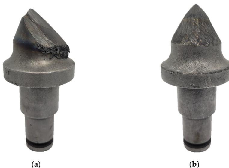
**Figure 1.** Tools with local cavities—(a); uniform abrasions—(b).
