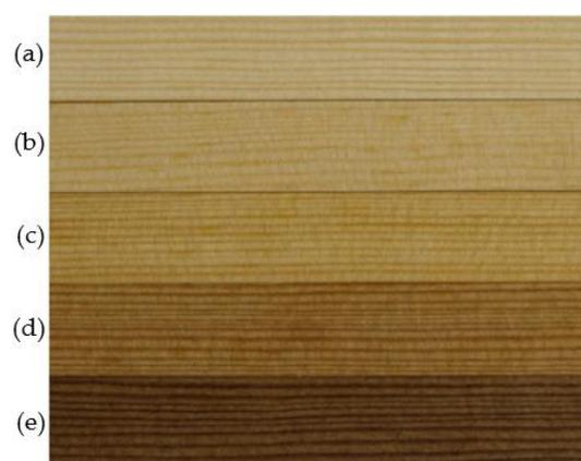
**Figure 2.** Sample surface—control (a) and modified wood (constant modification time—4 h) at a temperature of 130 °C (b); 160 °C (c); 190 °C (d); 220 °C (e).
