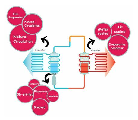
Figure 1. Categorization of different components of an LHP system based on wick structures, evaporators, and condenser.
