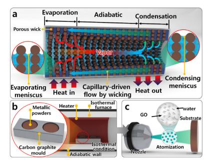
**Figure 7.** (a) Schematic of a heat pipe with a two-phase flow loop, (b) sinter of non-uniform copper particles at 600 °C using an isothermal furnace under a vacuum, and (c) suspension of graphene oxides in distilled water and the process of spraying this solution on copper wicks [94].
